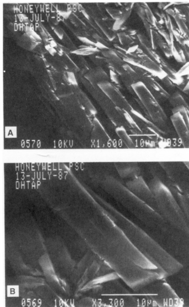
Figure 4. SEM micrograph of DHTAP/MSA crystallites.
